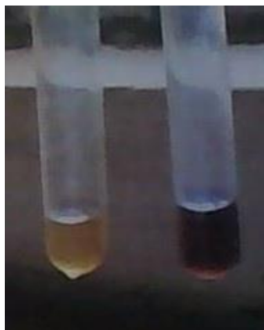
Plate I: Colour change from the ‘blank’ (test tube A) and the ‘test’ sample (test tube B) for the specific PA test using Ehrlich reagent
